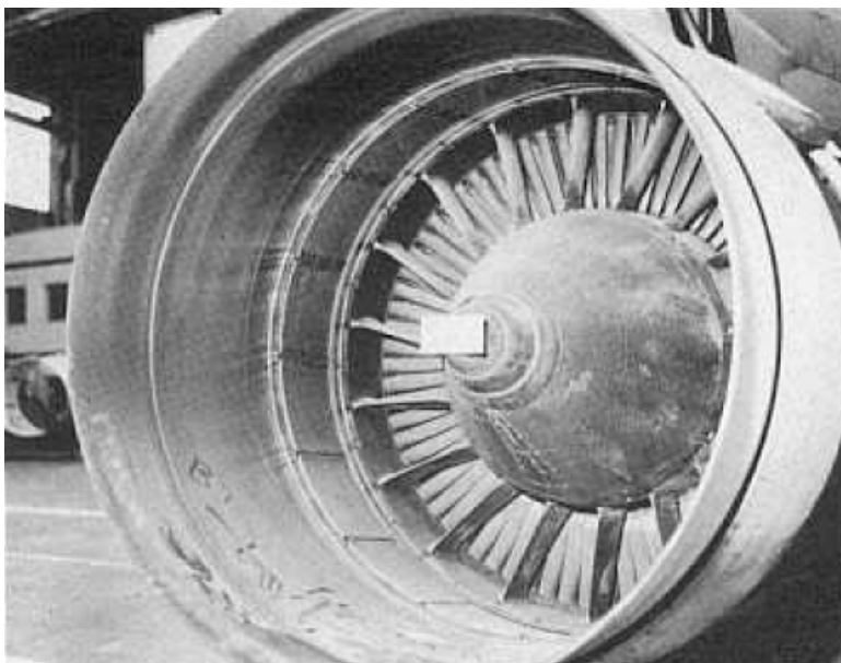
Figure 28: Engine Nacelle and nose cone stripped of paint.
