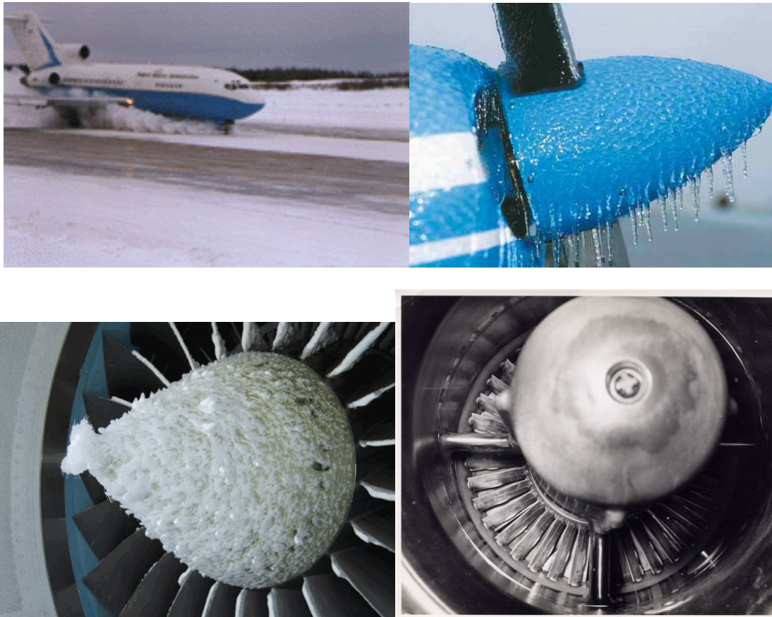
Figure 35: Severe ice accretion of aircraft and engines.
